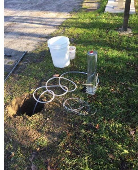
Figure B15. An example of the Constant-Head Borehole Permeameter Test in progress using a Johnson Meter.
