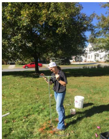
Figure A20. A hand auger was used to assess soil conditions and infiltration potential at Currier Park.
