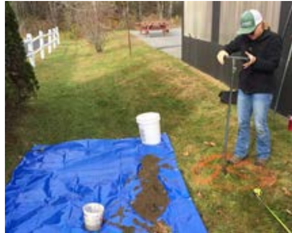
Figure B12. Soil testing was completed adjacent to the Wilkins Harley Davidson parking lot to confirm soil infiltration potential.
