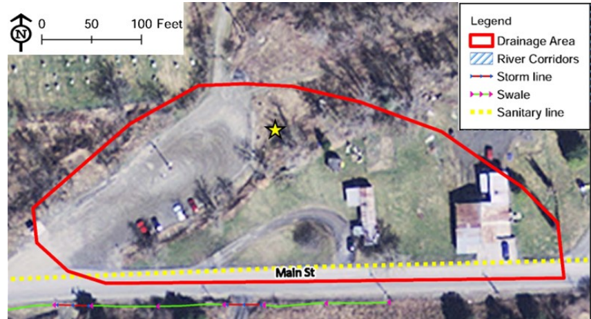
Figure C16. A gravel wetland is proposed to manage drainage from the Plainfield Park and Ride and surrounding area. The recommended location is shown with a star.
